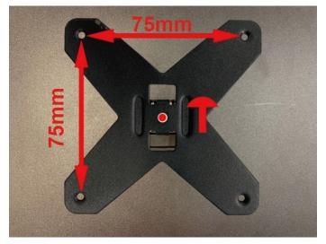
2. Once the stand is removed, you will see the indentation where you can install the mounting plate. The mounting pattern is 75mm x 75mm using M4 x 10mm screws.
