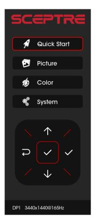
When you press the  $\checkmark$  button on the monitor, the OSD screen will appear. Select each of the functions with the  $\uparrow$  or  $\checkmark$  buttons. Use the  $\checkmark$  button again to enter each of the functions, or when you are in the function already, use the  $\checkmark$  button to select the option you want to adjust. Use the  $\uparrow$  or  $\checkmark$  buttons to adjust each option's values. When you want to exit, press the  $\overleftarrow{\frown}$  button.
