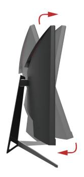
The screen can be adjusted by inclining forward and backward; however, the specific adjustment depends on the particular model of the device. Generally, it may be inclined  $5^{\circ} \pm 1^{\circ}$  forward and  $15^{\circ} \pm 2^{\circ}$  backward.
