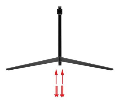
2. Install the assembled stand to the back of the monitor and screw in the 1 neck screws to secure the stand to the monitor.
